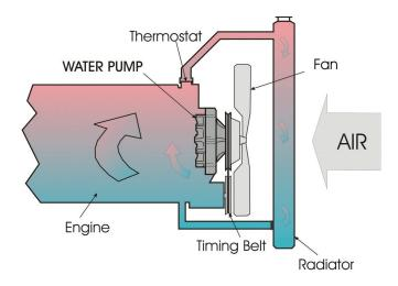
As coolant flows through the system, it picks up heat from the engine before arriving at the **thermostat**. The thermostat is a valve that measures the temperature of the coolant and opens to allow hot fluid to travel to the radiator. If the thermostat becomes 'stuck' and quits working, it will affect the entire cooling system.
